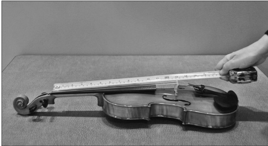
Figure 5-6: Measuring the vibrating length of the A string.
